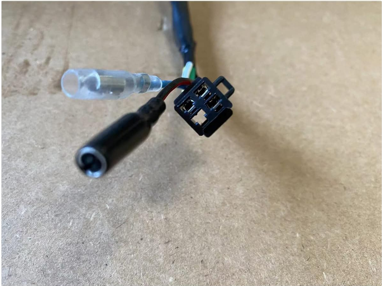
Figure 7: Close-up of the main wiring harness connector, essential for electrical connections.
