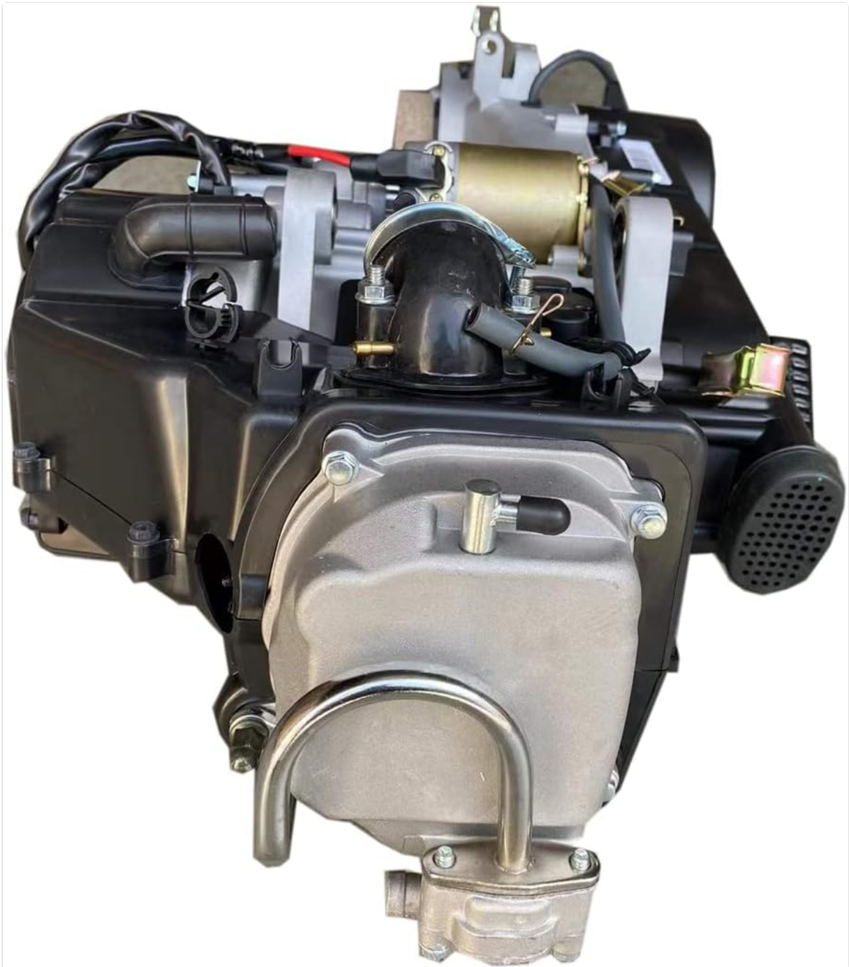
Figure 6: Front view of the X-PRO 150cc GY6 engine, showing the cylinder head and intake manifold area.
