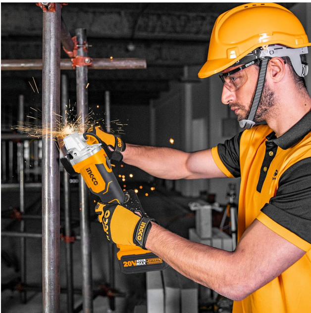
Cutting a metal pipe with the angle grinder.
