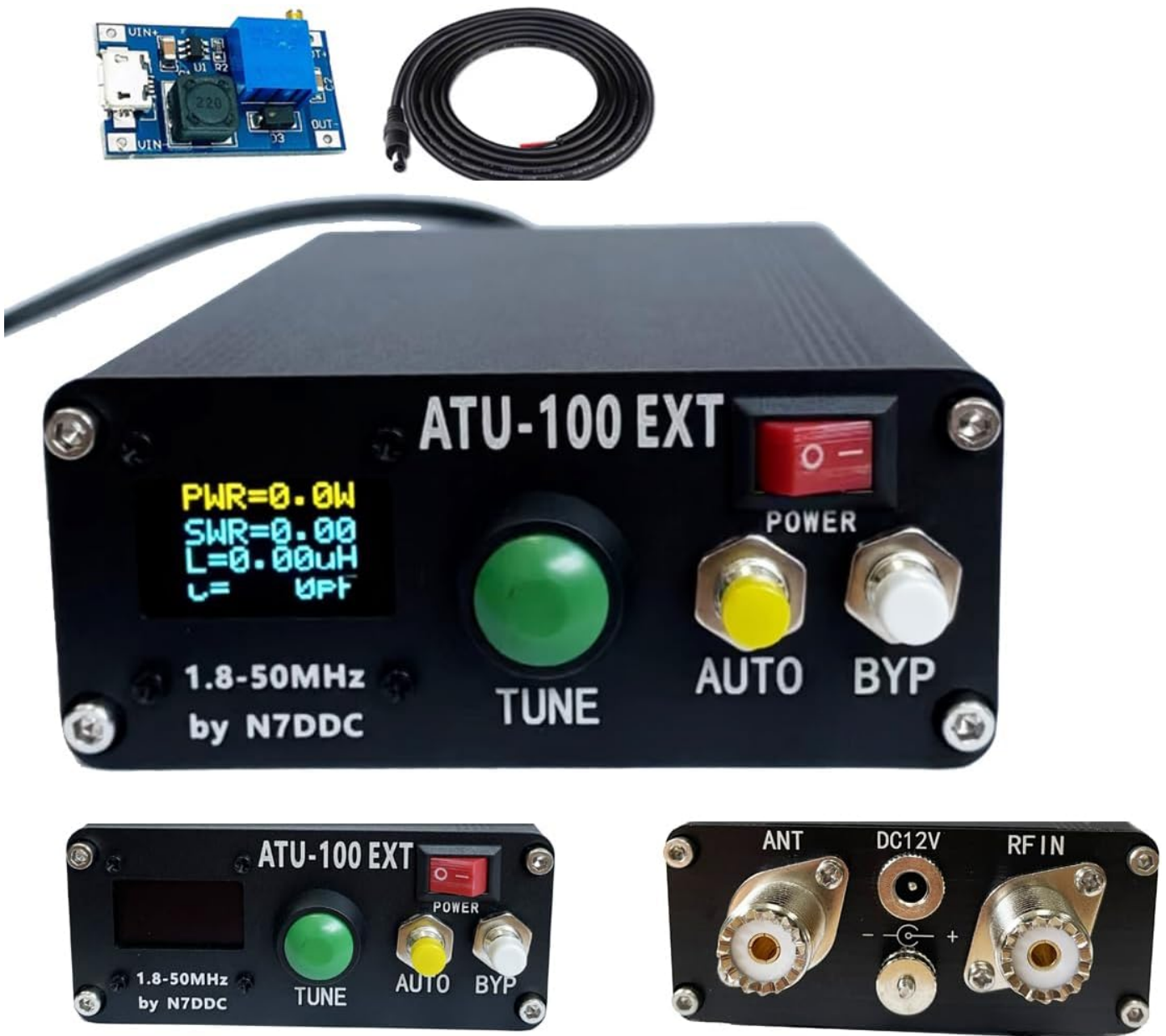
Image: Front view of the ATU-100 tuner, showing the display, Tune button, Auto button, BYP button, and Power switch.
