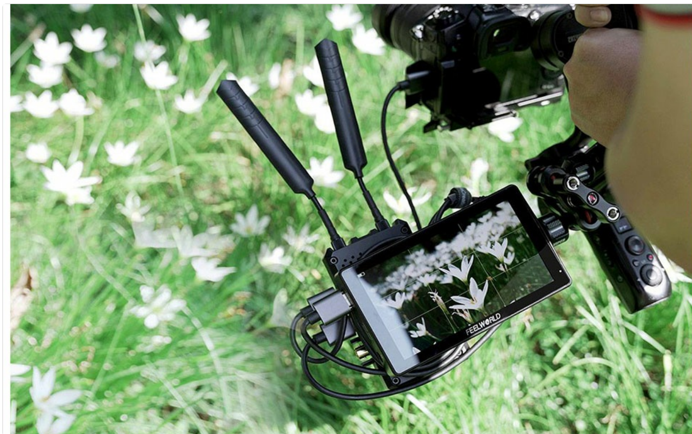
Image: The LUT5 monitor mounted on a camera setup, illustrating its integration with a wireless video transmitter for professional use.
