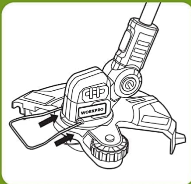
③ Attach the flower guard to the motor housing
