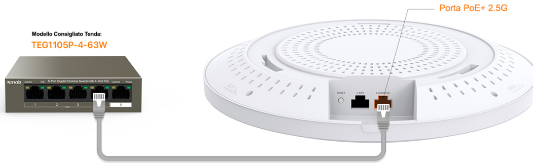
Image: Diagram illustrating PoE+ connectivity, showing the Tenda BE5010 connected to a PoE+ switch via a single Ethernet cable for both power and data.
