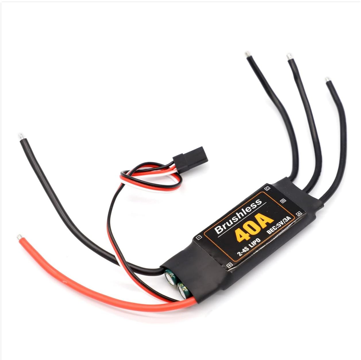
Figure 2: Overview of the RUIZHI 40A ESC, showing the main body, battery input wires (red and black), motor output wires (three black wires), and the signal wire with a servo connector.
