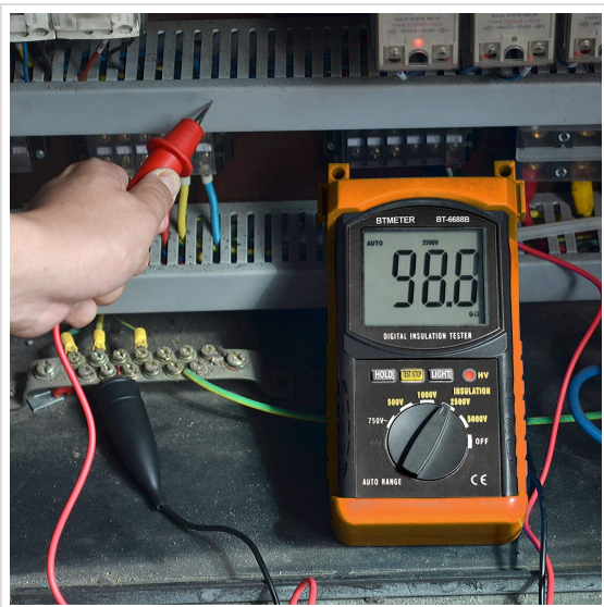
Figure 5.1: The AP-6688B being used to measure insulation resistance in an electrical panel.
