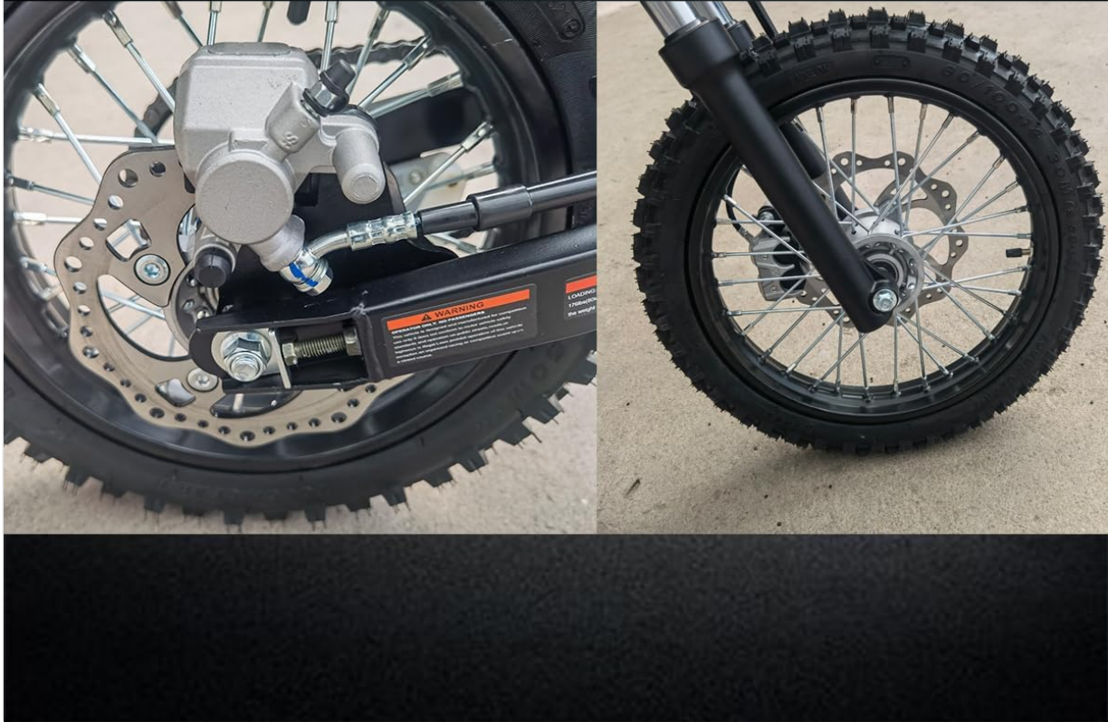
Image: Close-up view of the front and rear hydraulic disc brakes on the X-PRO X27, providing superior stopping power and control.
