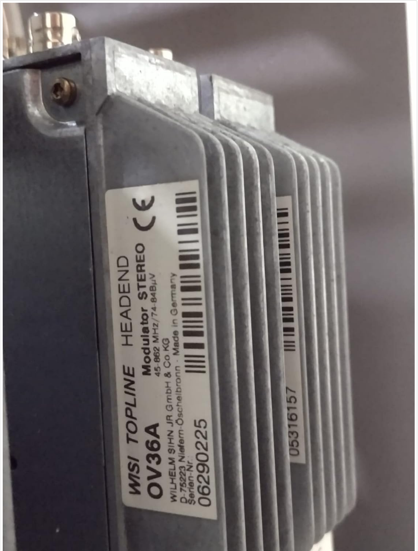
Figure 4.2: Close-up of the side label of a WISI TOPLINE OV36A Headend Modulator Stereo module. This label provides model information, frequency range (45-862 MHz), and serial numbers like 05316157 and 06290225, indicating manufacturing details.
