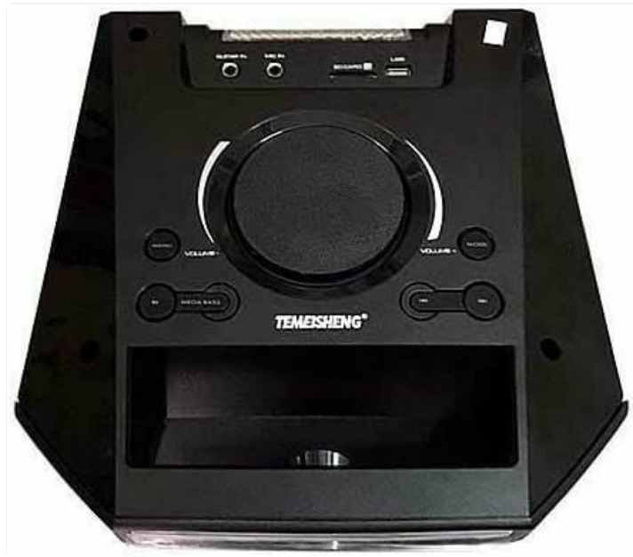
Figure 1: Top Control Panel of the TMS-802 Speaker. This image displays the main rotary volume knob, smaller volume controls for microphone and echo, input selection buttons, and ports for USB and SD card.
