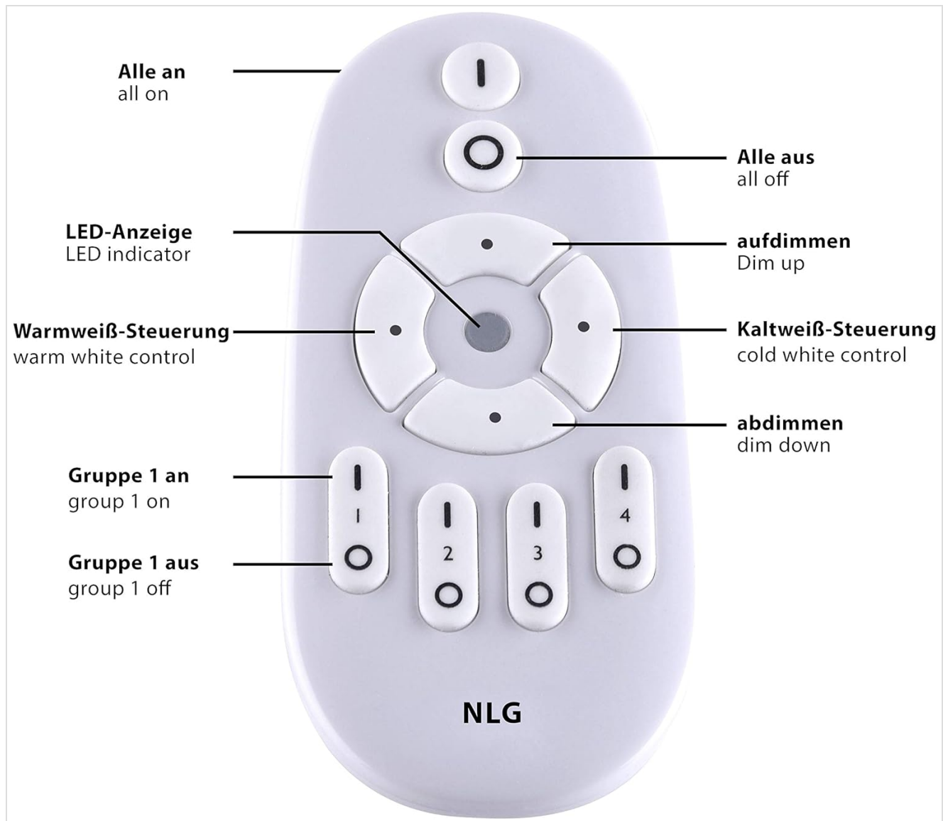
Figure 5.1: The wireless remote control for the LED ceiling panel, showing buttons for power, dimming, color temperature adjustment, and group control.
