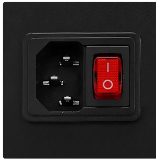
Figure 8: Power switch. This image shows the main power switch located on the rear panel of the chiller unit.
