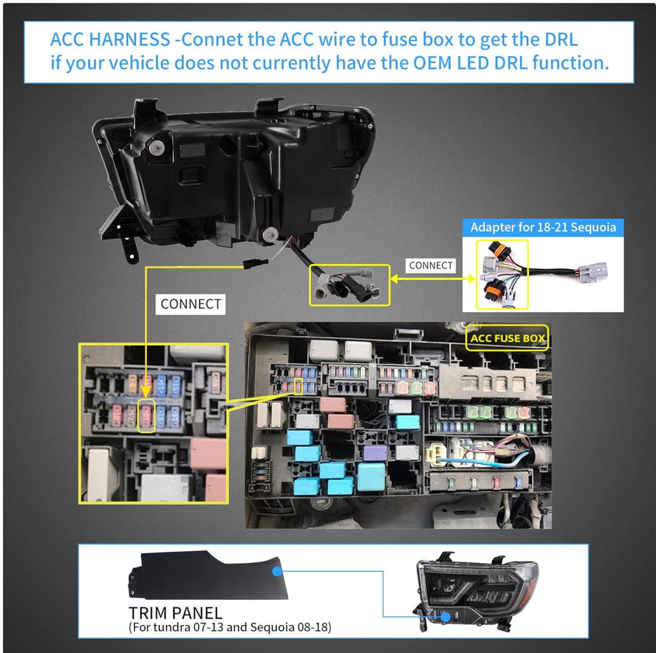
Image 4.2: Wiring diagram illustrating the connection of the ACC harness to the vehicle's fuse box for DRL functionality and the placement of the trim panel.
