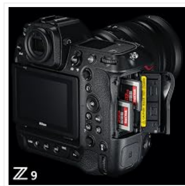
Figure 3.1: Memory card slots of the Nikon Z 9, illustrating proper card insertion.
