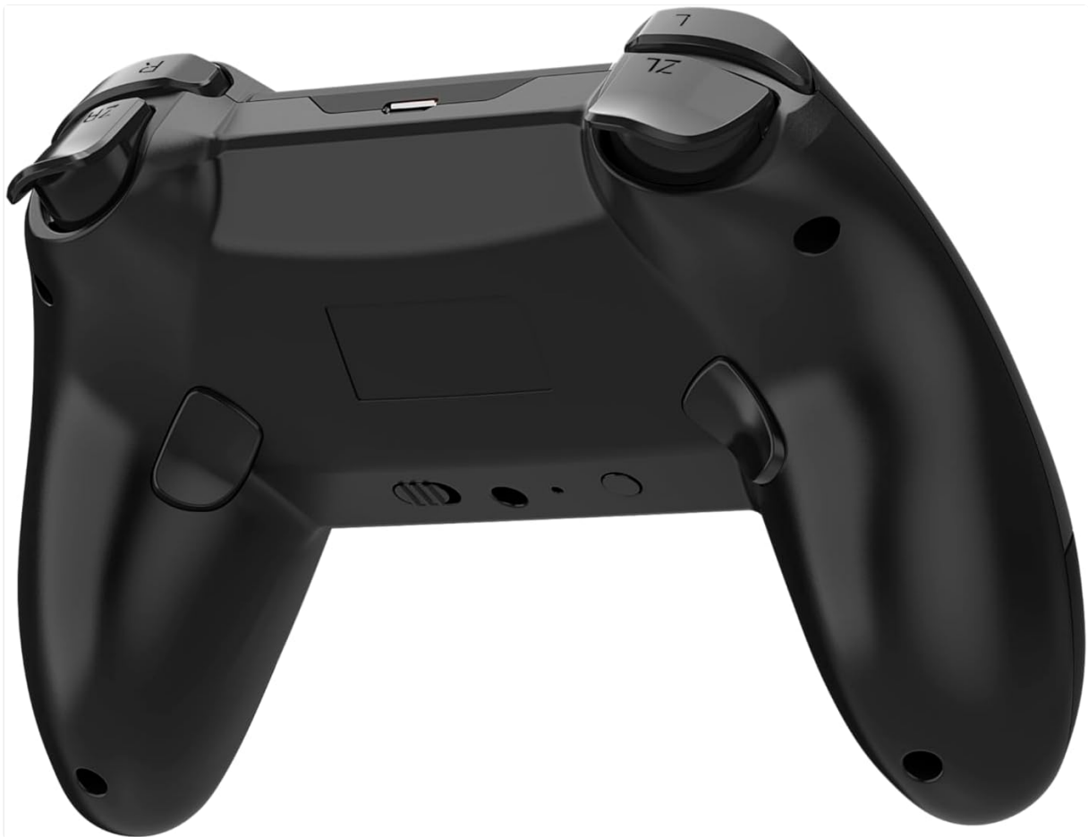
Figure 3: USB-C Charging Port Location. The port is located on the top edge of the controller.
