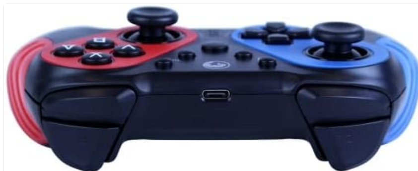
Figure 2: USB Type-C Charging Port. This image shows the location of the USB Type-C port on the top edge of the controller, used for both charging and wired connection.
