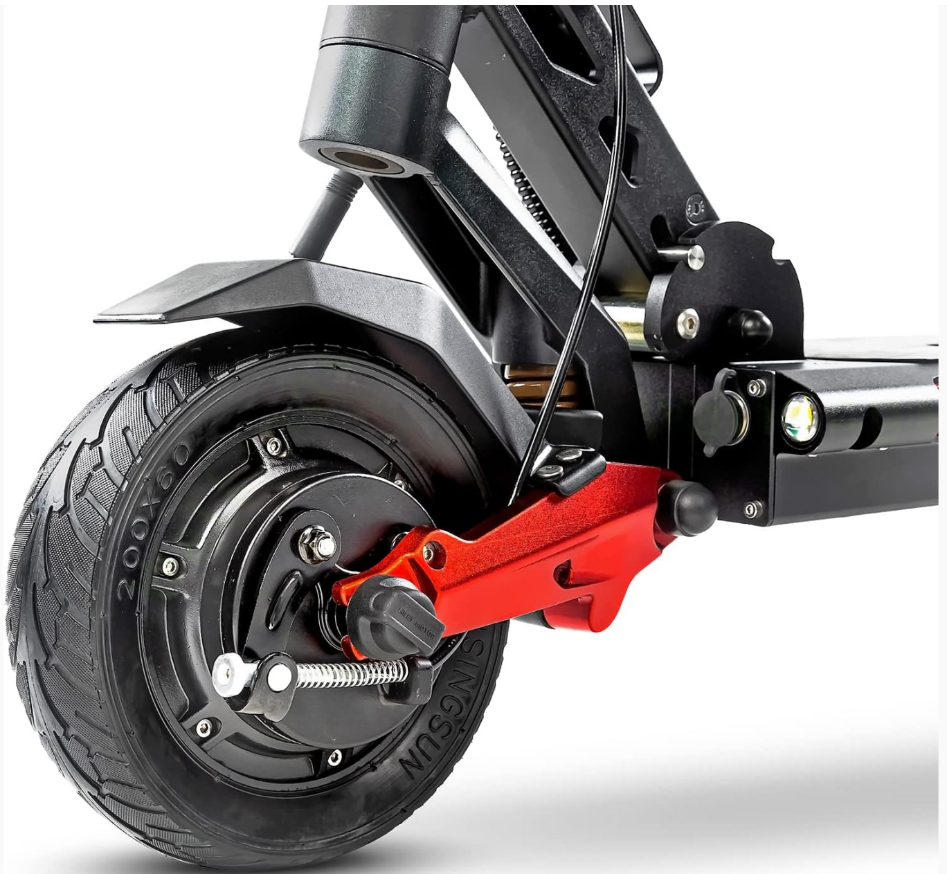
Image: Detail of the front wheel assembly, highlighting the hydraulic disc brake and high-performance suspension.
