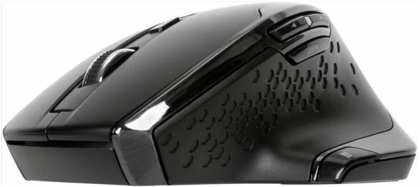
Figure 5.1: Angled view of the mouse, highlighting the placement of the side buttons and the textured grip area.
