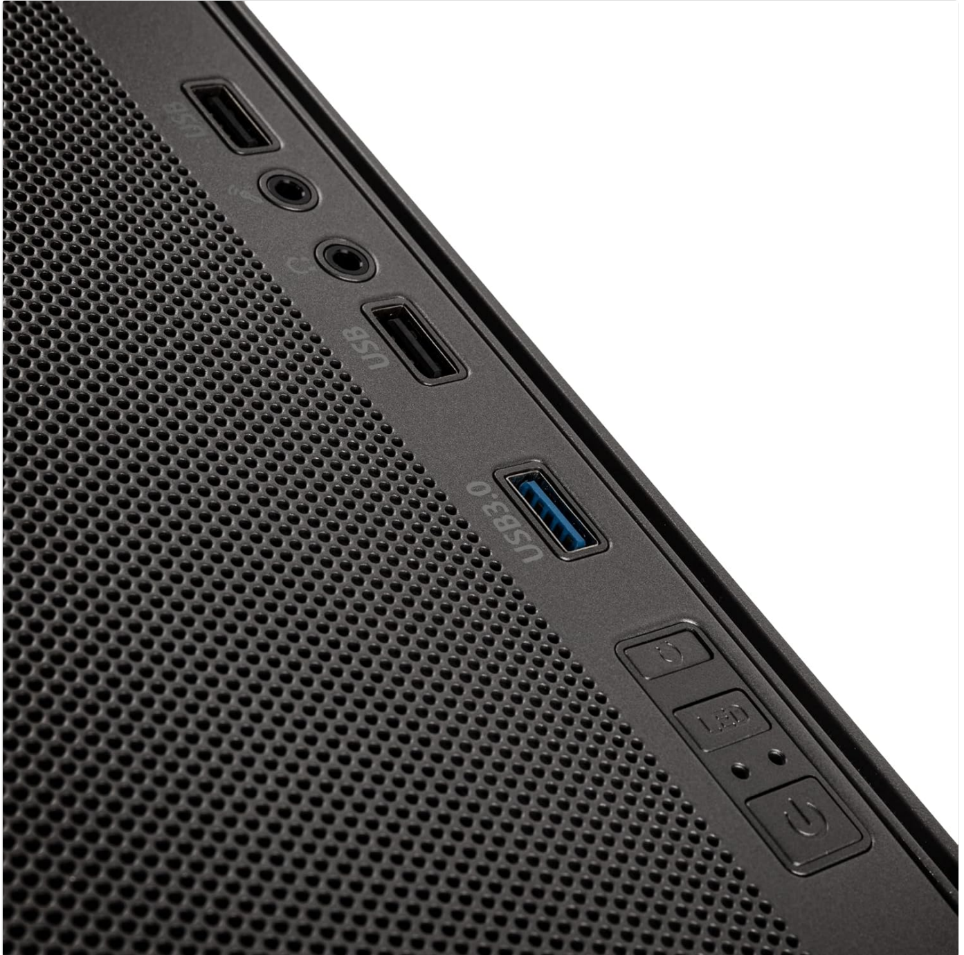
Image: Close-up view of the top I/O panel, showing the USB 3.0, USB 2.0, audio jacks, and power/reset buttons.
