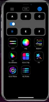
Figure 7: The app's group control interface, illustrating how multiple lights can be managed for synchronized or varied lighting effects.
