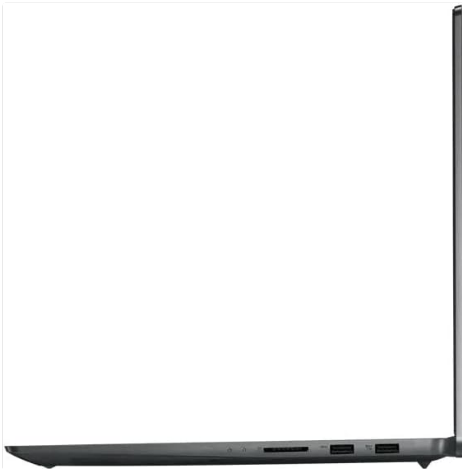
Image: Right side of the laptop, displaying USB 3.0 ports and an SD card reader slot.
