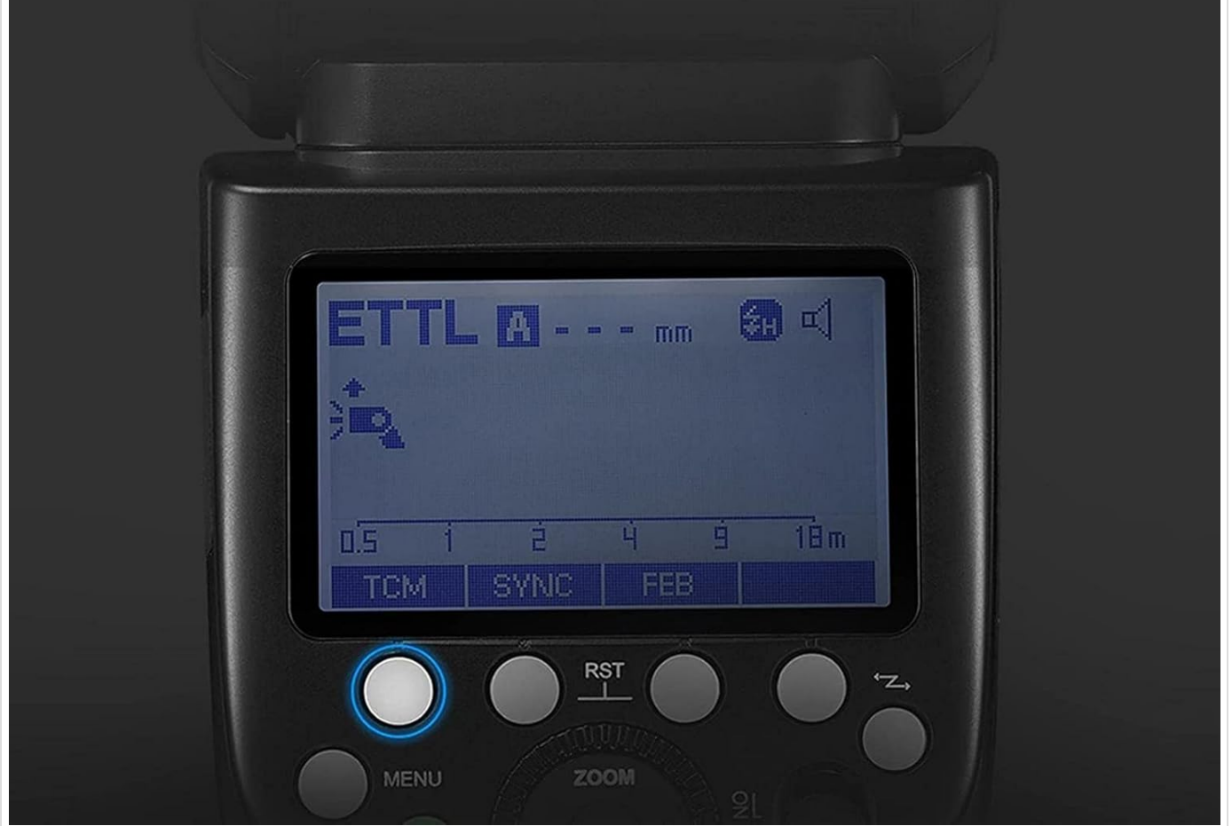
Image: The LCD display of the Godox TT685II-C, highlighting the TCM (TTL Converted to Manual) function button.
