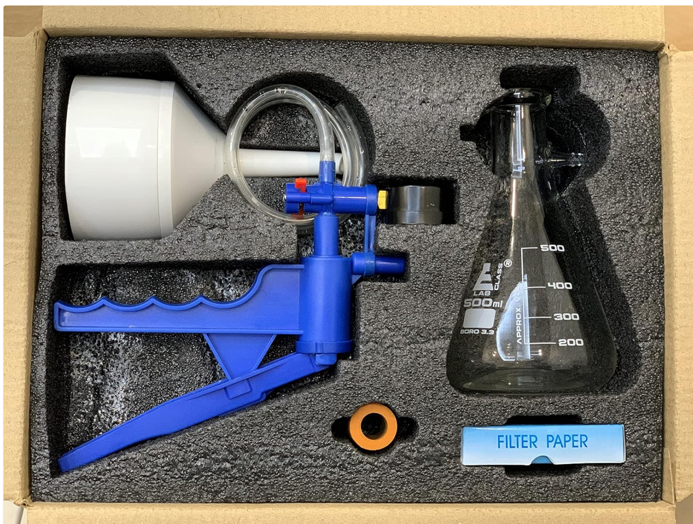
Image: The EISCO Vacuum Filtration Kit components neatly organized within their protective foam insert, as received in the packaging.
