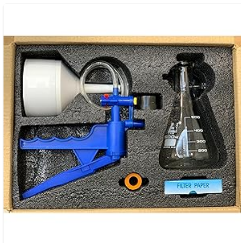
Image: A labeled diagram illustrating each component of the vacuum filtration kit, including the Buchner funnel, rubber stopper, filtering flask, hand vacuum pump, flexible tubing, and filter paper.
