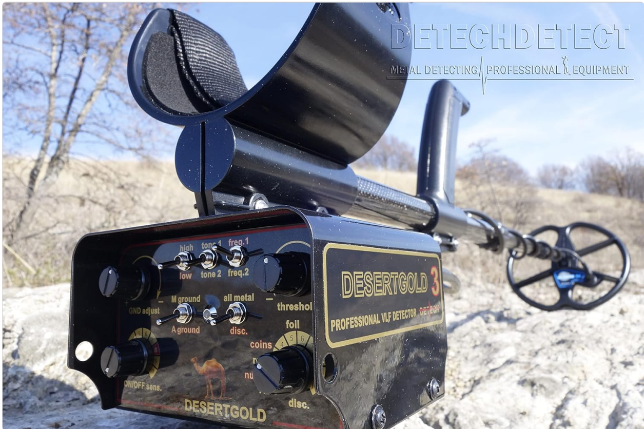
Image 3.1: Close-up view of the DETECH Desert Gold 3 control panel, showing various knobs and switches.
