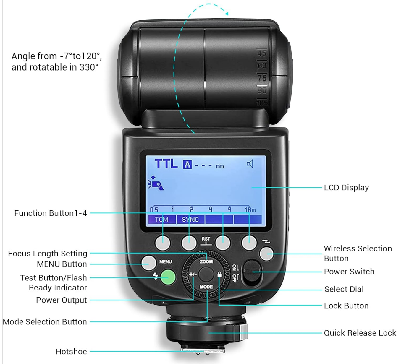
Figure 4: Control Panel Overview
