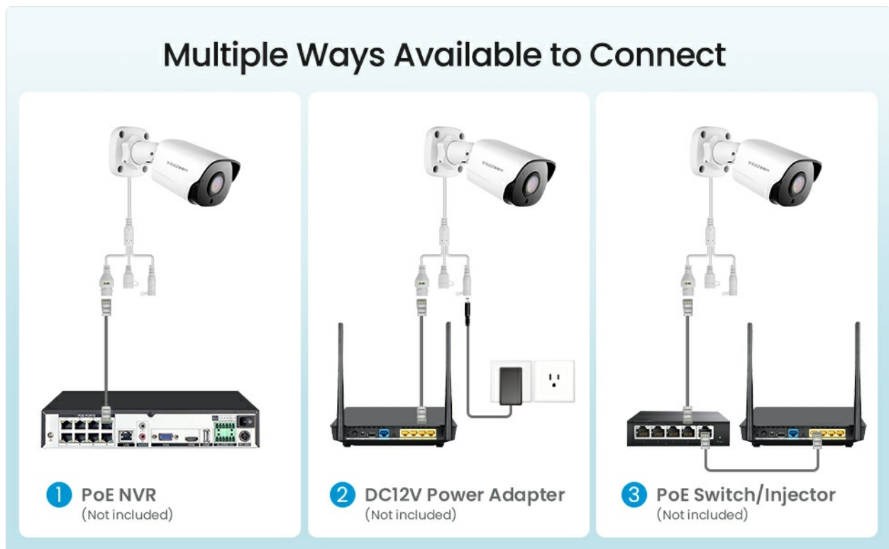
Image: Three connection diagrams illustrating how to connect the camera to a PoE NVR, a DC12V power adapter and router, or a PoE switch/injector and router.
