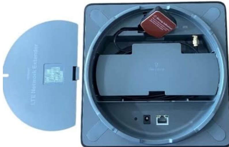
Figure 3.1: Bottom view of the Network Extender with the cover on, showing the Ethernet and power ports.
