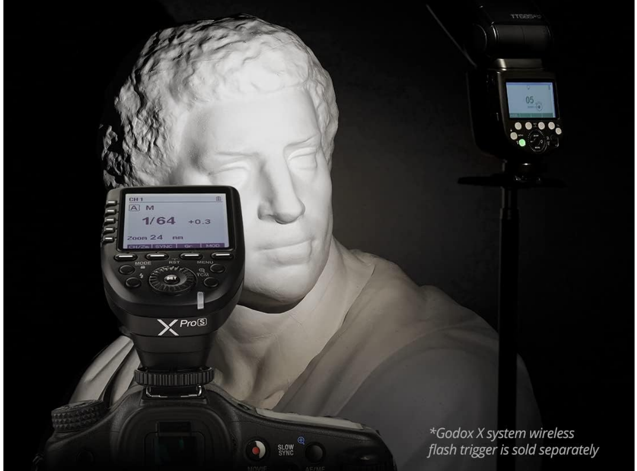
Figure 7: The Speedlite operating as part of the Godox 2.4G Wireless X System, allowing remote control and multi-flash setups. To select Transmitter (TX) or Receiver (RX) unit, short press the Wireless Selection Button . Ensure the channel and group settings match between the transmitter and receiver units for successful communication.
