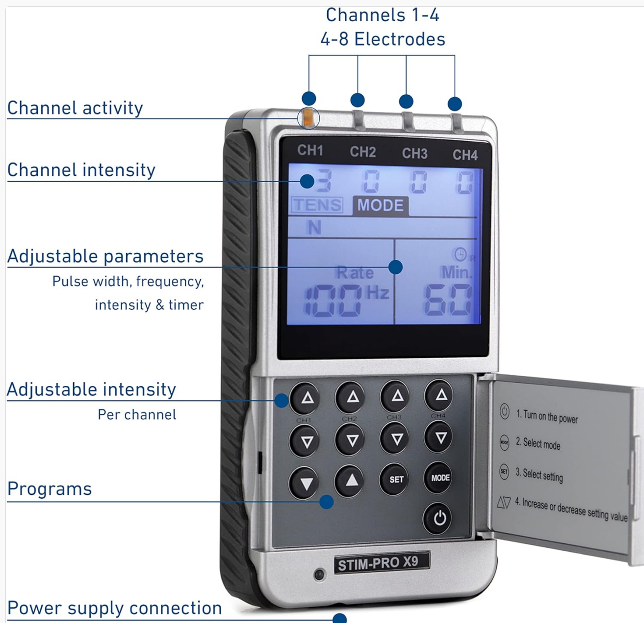
Image 4.1: Front view of the STIM-PRO X9+ with labeled controls and display elements.
