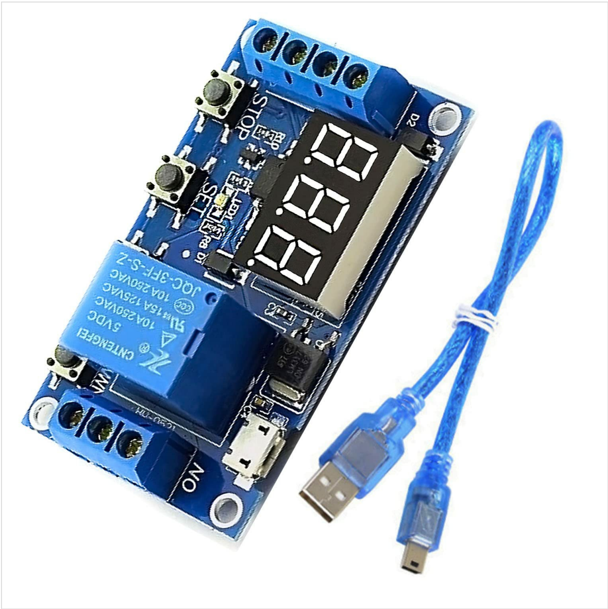
Figure 2.1: DEVMO JZ801 Relay Board and USB to Micro USB Power Line.
