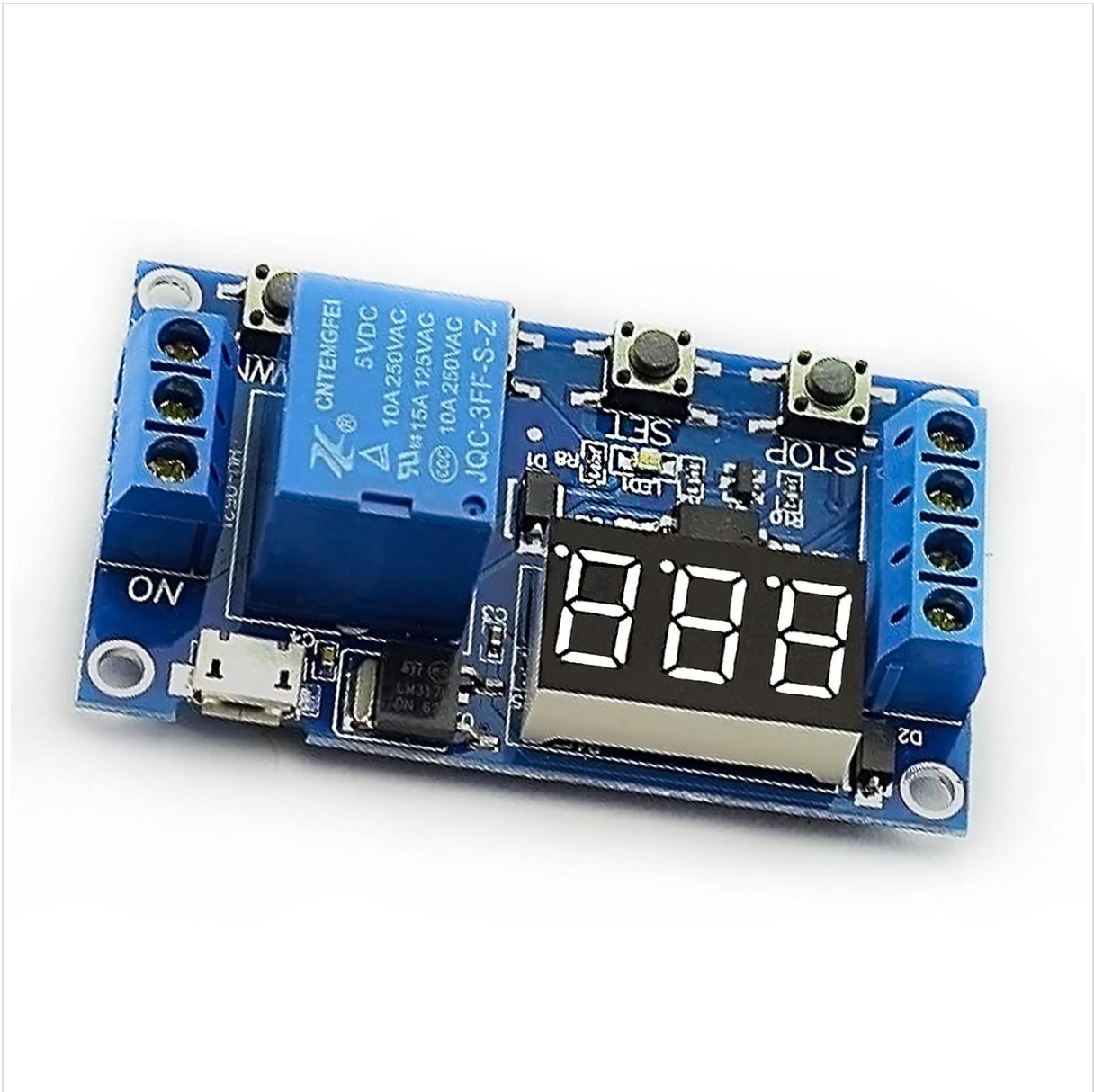
Figure 3.1: Top view of the DEVMO JZ801 Relay Board.
