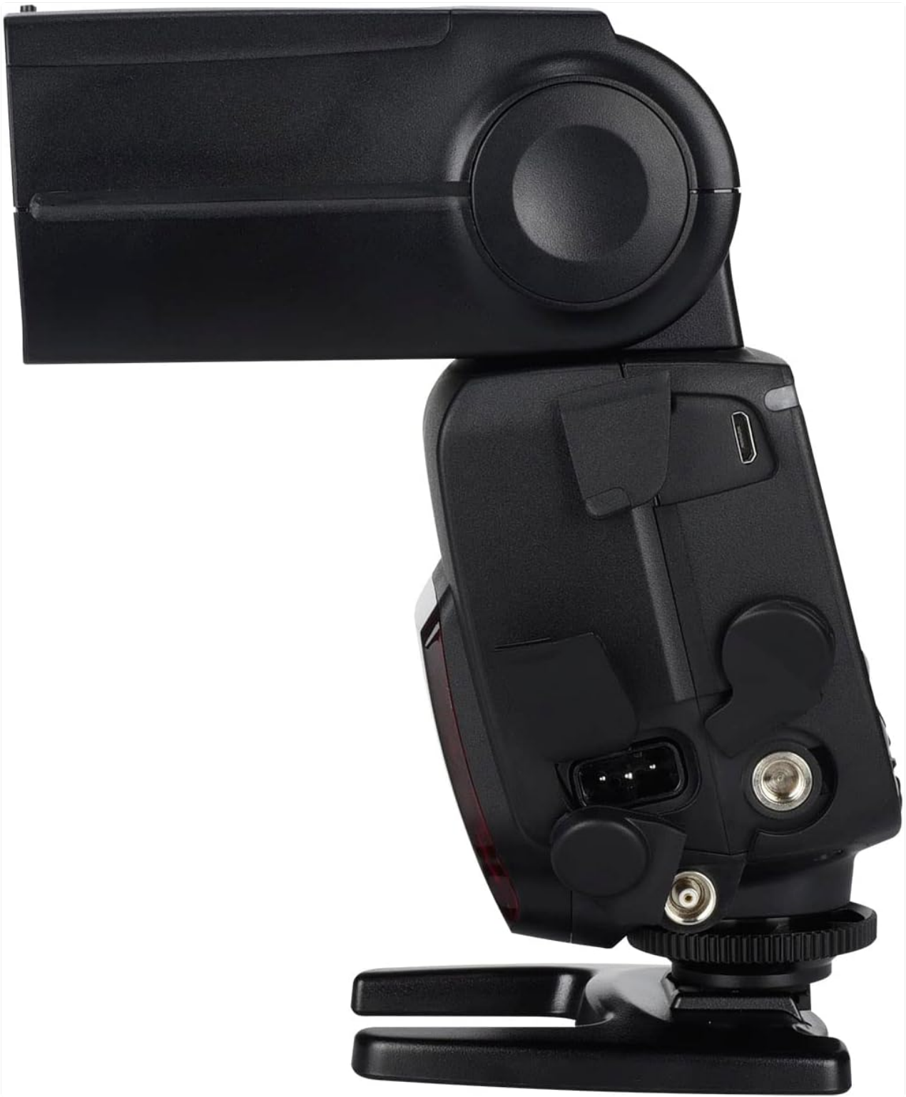
Image: Side view of the YN685EX-RF flash unit, highlighting the external power port and USB update port.
