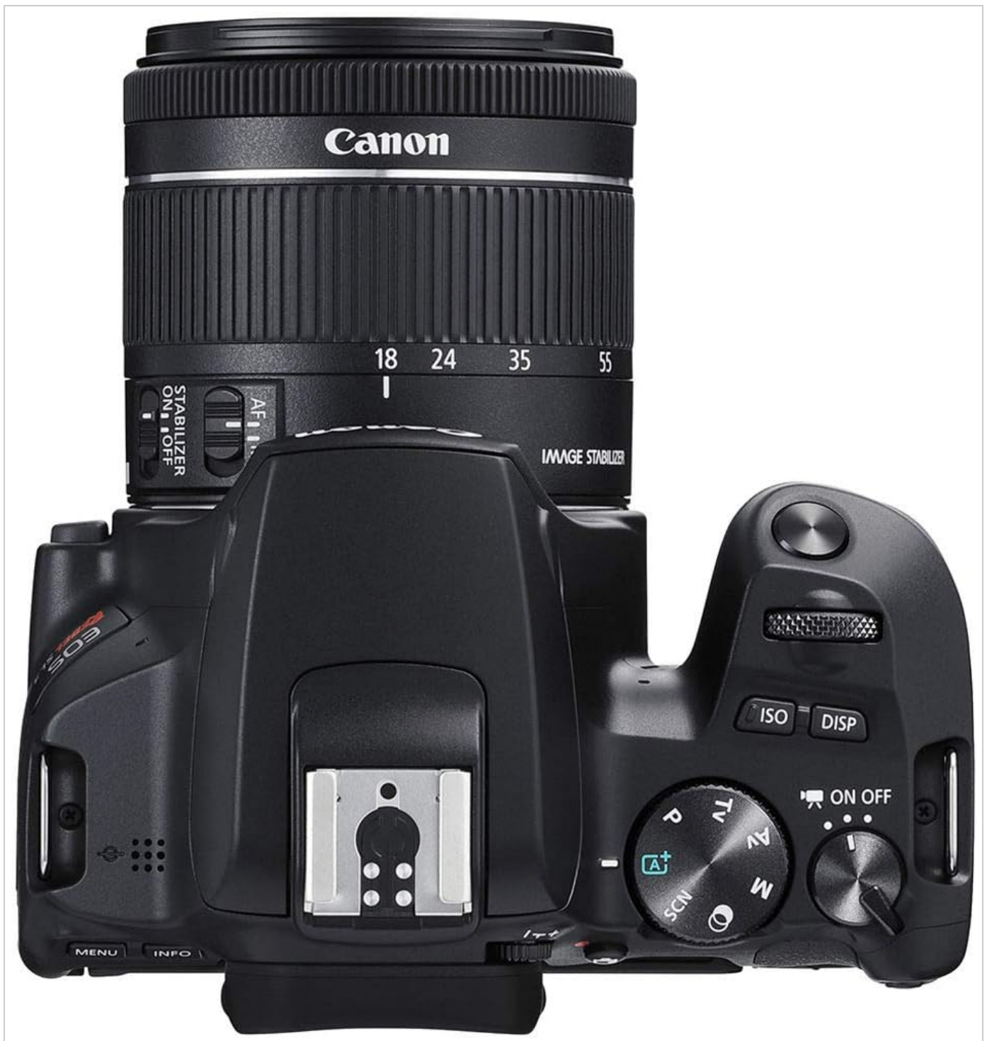
Figure 3.1.1: Top view of the Canon EOS Rebel SL3, highlighting the mode dial, power switch, and hot shoe.
