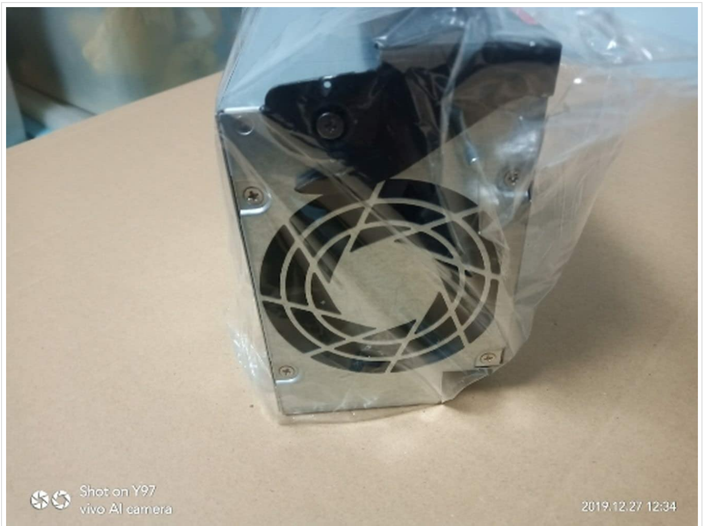
Figure 3: Close-up of the power supply's cooling fan.
