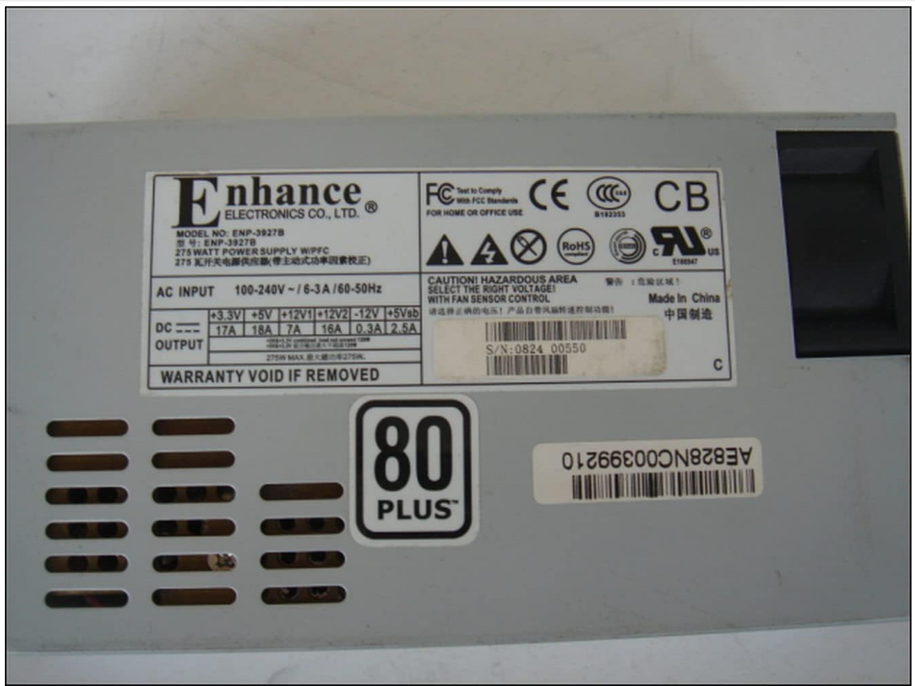
Image 2: Close-up of the power supply's label, displaying model number ENP-3927B, 275W rating, 80PLUS certification, and electrical input/output specifications.
