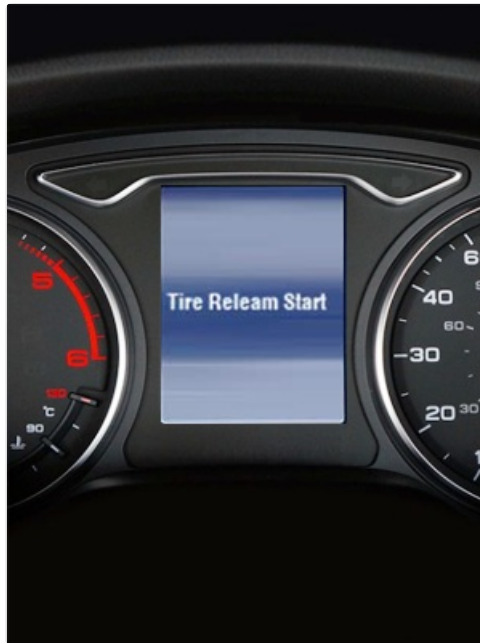
Figure 4: Example of a vehicle dashboard indicating the 'Tire Relearn Start' message.
