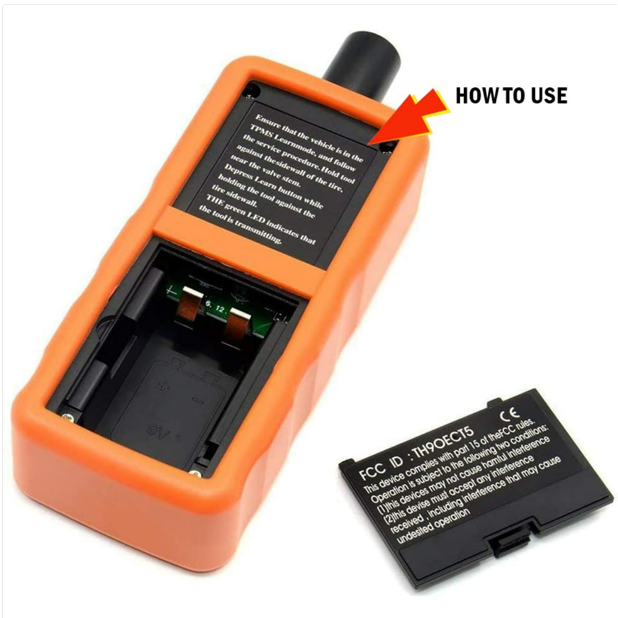
Figure 3: The EL-50448 tool with its 9V battery compartment open, showing where to insert the battery.
