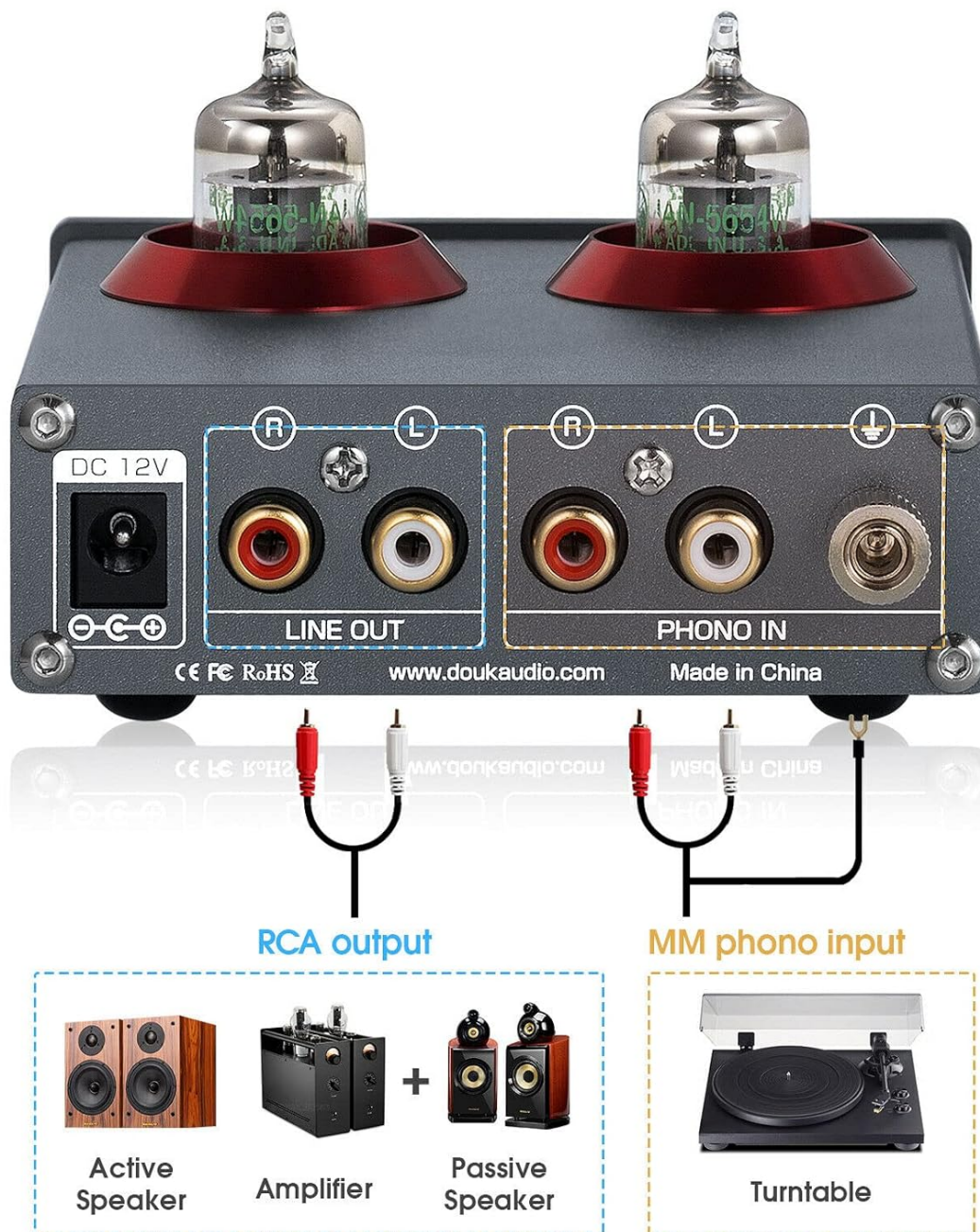
Figure 4: Rear Panel Connections (Power, Line Out, Phono In)
