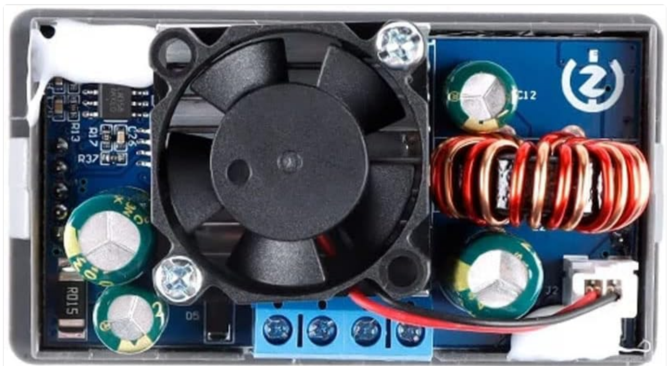
Figure 3.3: Internal view of the ZK-5KX module, showing the circuit board, heat sink, and integrated cooling fan for thermal management.
