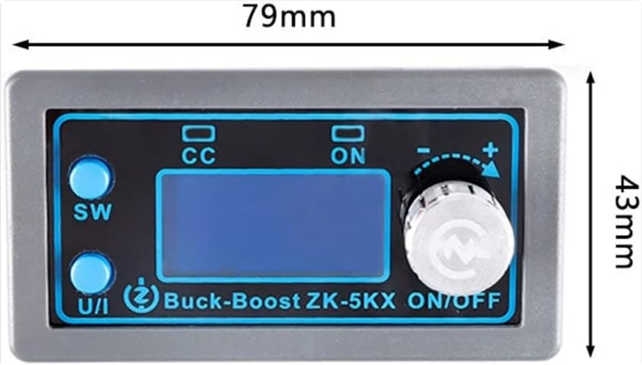
Figure 4.1: Dimensions of the ZK-5KX module, indicating a length of 79mm and a width of 43mm.
