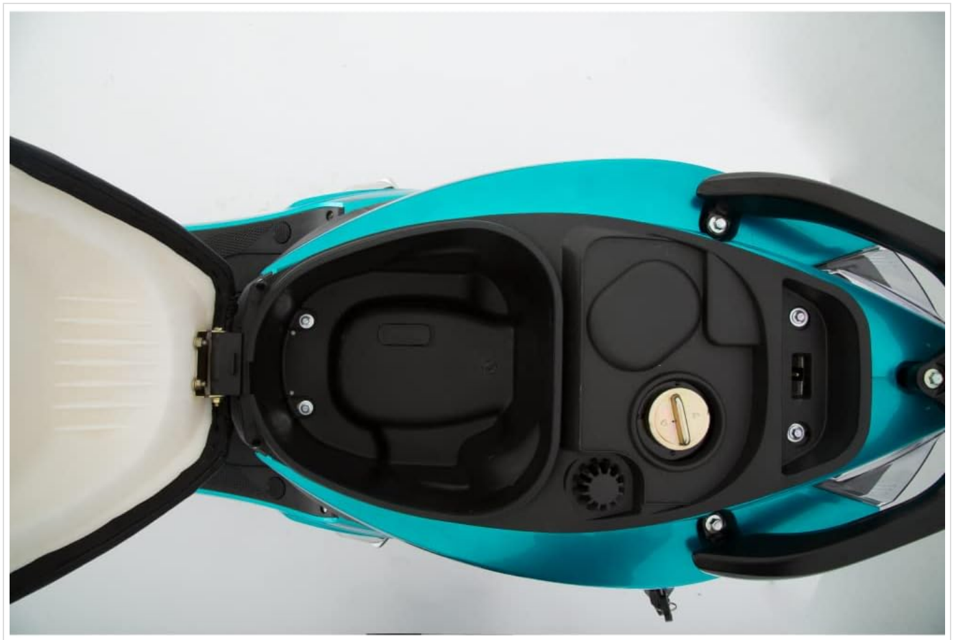
Image: View of the under-seat compartment, showing the fuel filler cap and storage space, essential for pre-ride checks and fueling.
