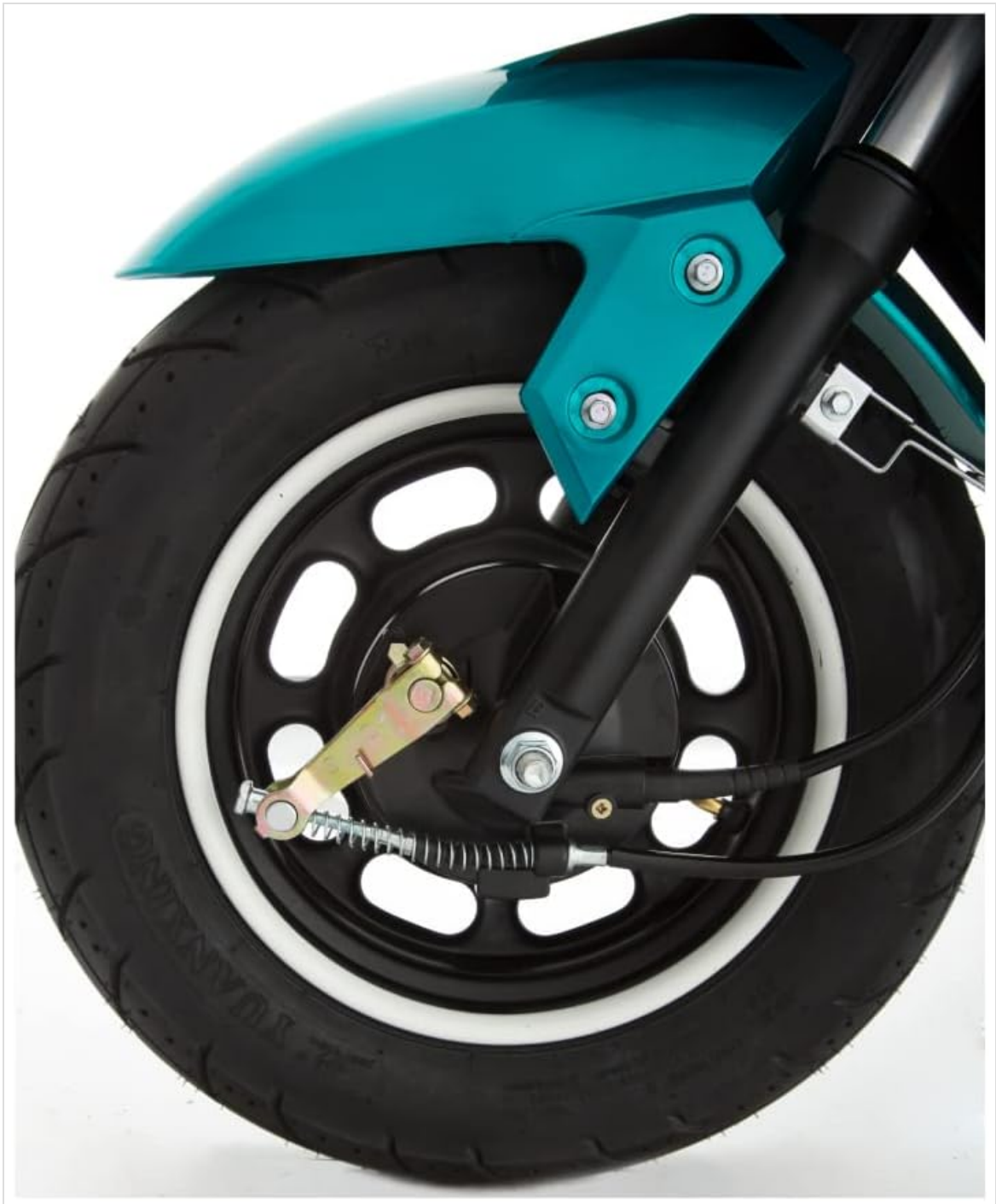
Image: Close-up of the front wheel and suspension system, highlighting the brake mechanism and tire tread, crucial for safety checks.
