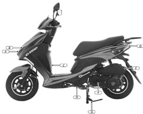
Image: Labeled diagram of the scooter, indicating key components such as (A) Front Headlight, (B) Front Turn Signal, (C) Serial Number Housing, (D) Rear Turn Signal, (E) Air Filter, (F) Kick Start Pedal, (G) Center Stand, and (H) Side Stand.
