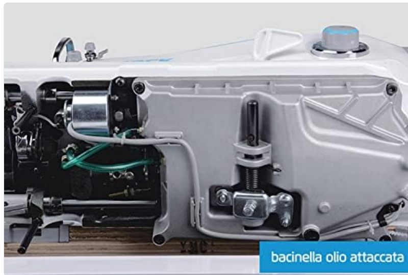
Figure 4.1: A detailed view of the machine's internal components, highlighting the oil basin ("bacinella olio attaccata") which is part of the automatic lubrication system. Regular checks of this system are recommended.
