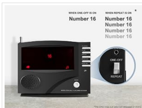
Image: The switch on the CMU to select between one-off and repeat alert modes.
