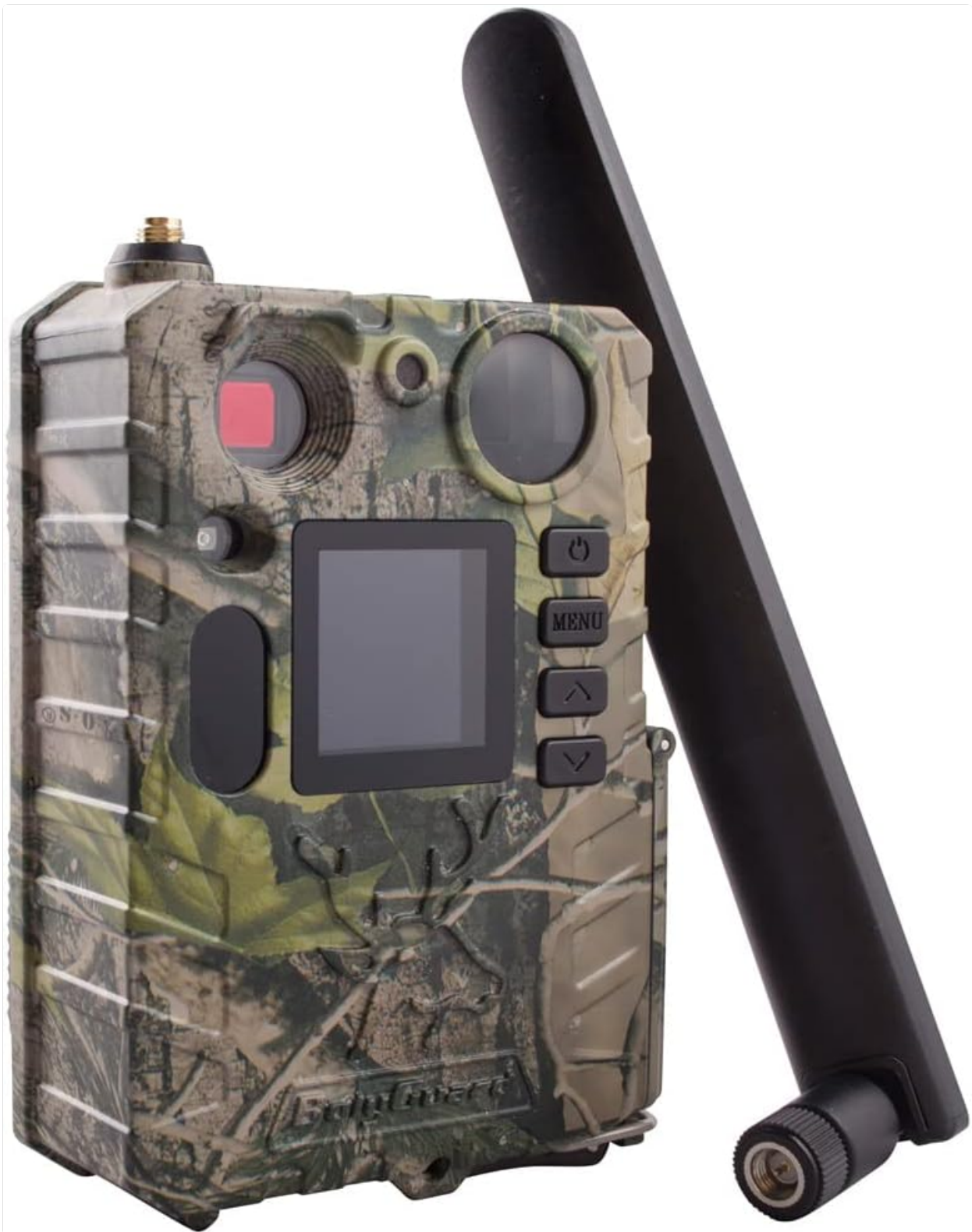
Image 2.3.1: Front view of the Bolyguard BG710-M Trail Camera. The image shows the camouflage-patterned camera body, the lens, infrared LEDs, motion sensors, control buttons (Menu, Up, Down, OK), and a small display screen. A black antenna is attached to the top right side.
