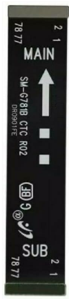
Figure 1: Vertical view of the Ygpmoiki Main Flex Cable, indicating main and sub-connections.
