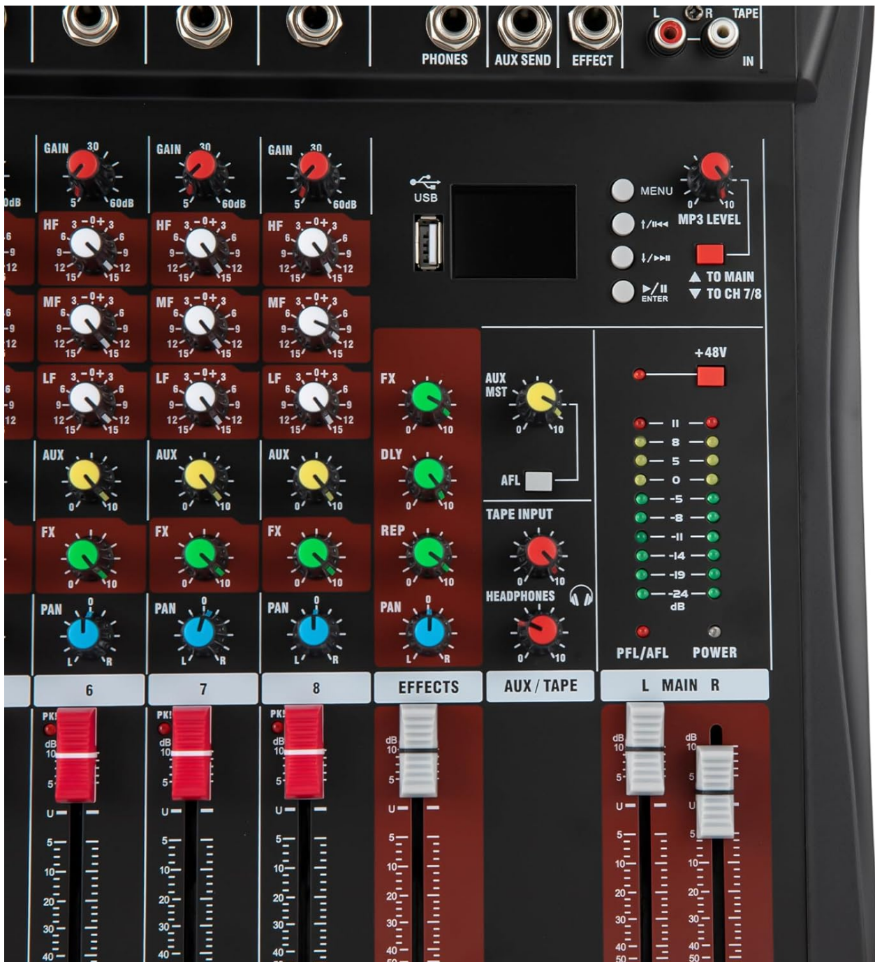
Figure 6: The master control section, featuring USB/MP3 player controls, effects parameters, AUX/Tape input, headphone volume, and main output level meters.
