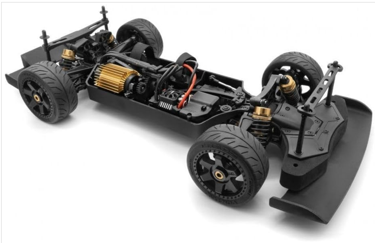
Figure 4: Underside view of the Maverick QuantumR Flux 4S Race Truck chassis, showing the motor, ESC, and drivetrain components.
