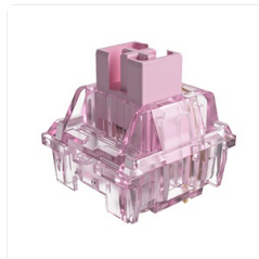
Image 4.1: A Jelly Pink mechanical switch, illustrating the hot-swappable design.
