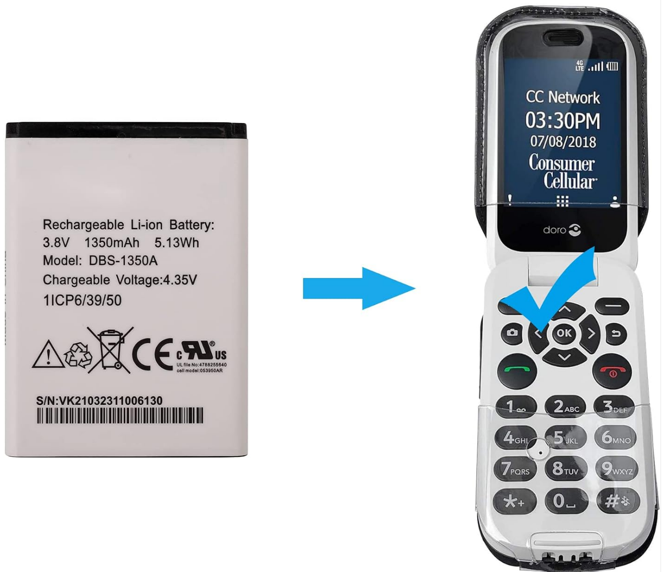
Figure 3.3: DBS-1350A battery shown with the compatible Doro 7050 phone.
