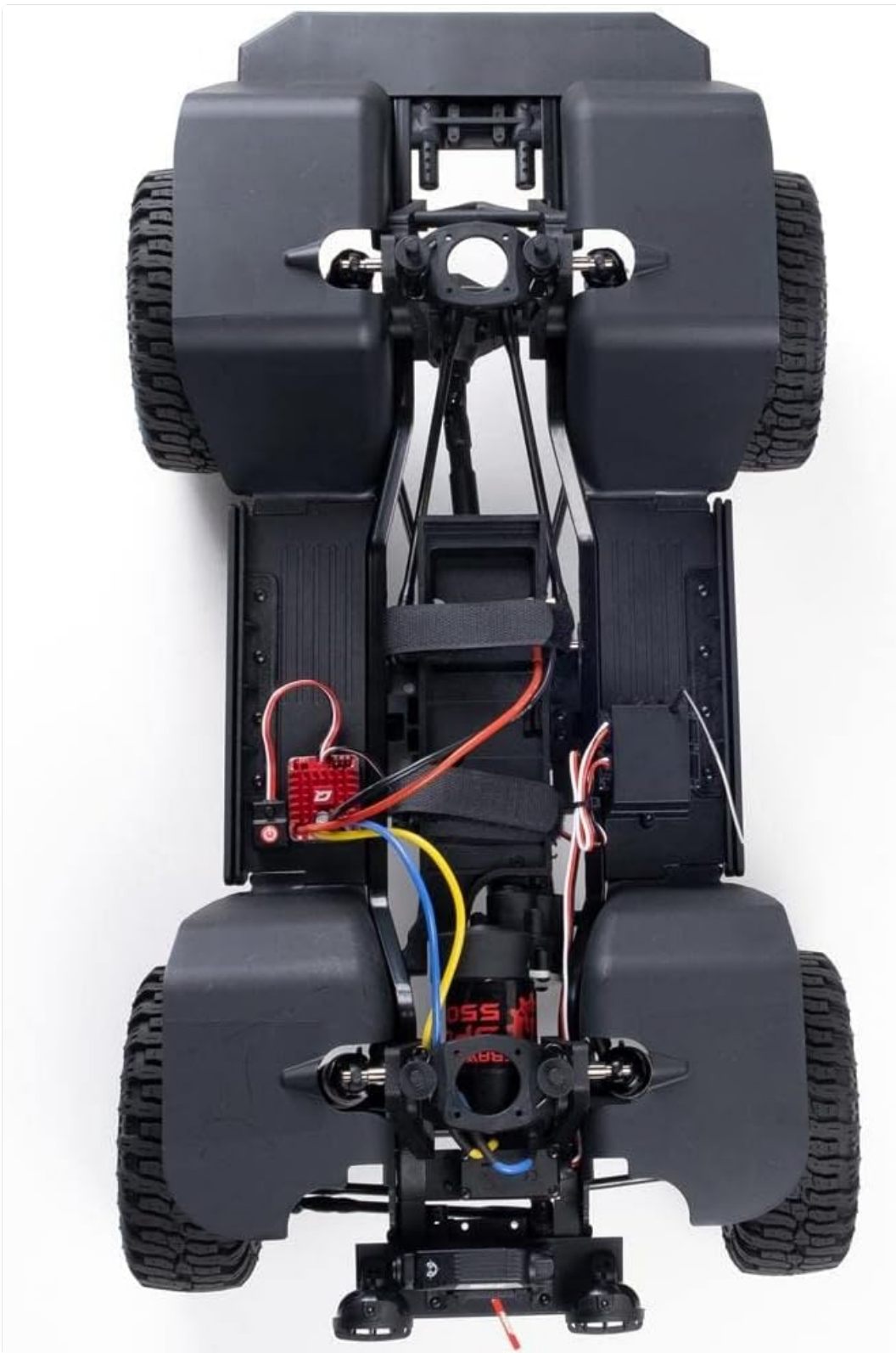
Figure 2.1: The underside of the TC8 Marksman, revealing the chassis and electronic components.
