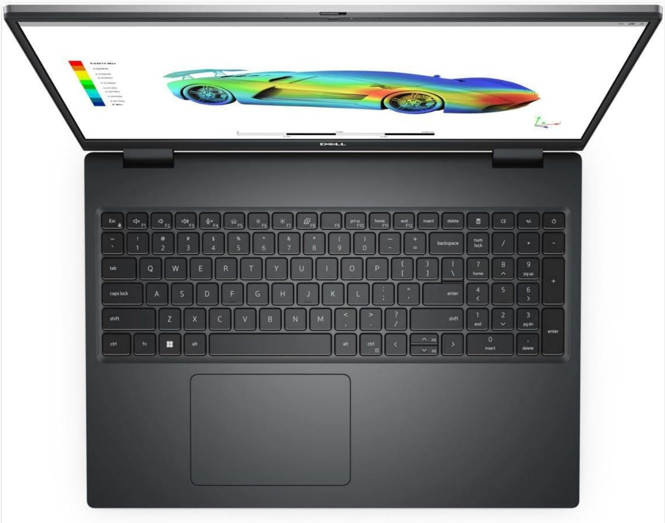
Figure 2: Top-down view of the Dell Precision 7670 keyboard and touchpad. This image highlights the full-size backlit keyboard with a numeric pad and the large, responsive touchpad.
