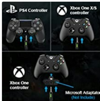
Image: Diagram illustrating how to connect the headset to an Xbox One controller, highlighting the need for a Microsoft adapter for older controllers.
