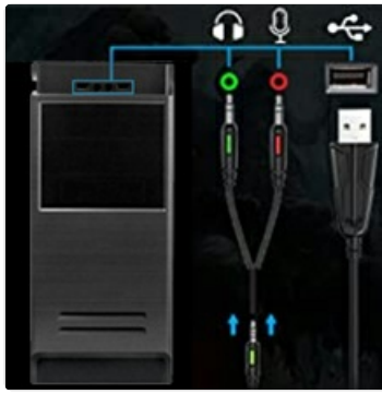
Image: Diagram showing the connection of the headset to a PC using the 1-to-2 splitter for audio and microphone, and a separate USB connection for LED lighting.
